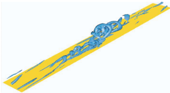
Fig. 3. The hairpin vortex packet that evolves in Re_t = 300 channel flow from the slightly asymmetric primary hairpin in Fig. 2. t^* = 250 . Note the complexity of this packet relative to the packet in Fig. 1. An animation of the evolution from the initial disturbance can be seen at http://www.ltcf.tam.uiuc.edu . The surfaces are contours of the swirling strength.
